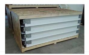
Doors are made to individual order specifications. After doors are completely assembled they are packaged in wood "surround". Doors are skidded up to four (4) high on 3070's and 4070's and two (2) high on 6070's. Skids are 4-way and have 4 length long runners.
